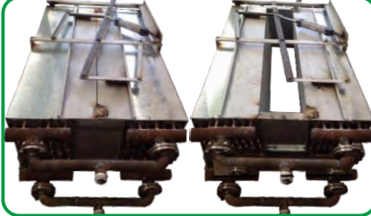
Heat exchanger for cool down dryer 打冷风
